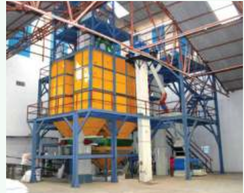
4-6 MT/hr Fully Computerised Automatic Pellet Feed Plant
