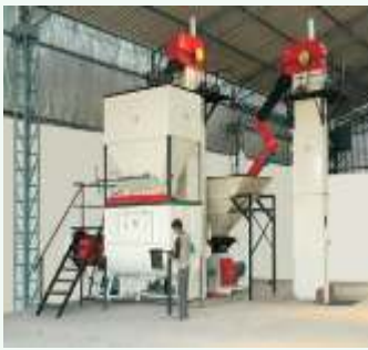
4-6 MT/hr Mash Feed Plant
